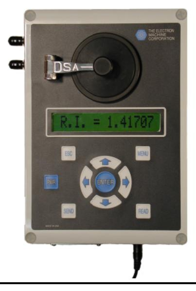
The DSA E-Scan is an automatic, benchtop critical angle refractometer with a digital readout and temperature-controlled sample chamber. It measures the critical angle of refraction of sample fluids which are directly correlated to various measurements including percent dissolved solids, Brix, and refractive index. The instrument is equipped with a menu-driven user interface and is factory calibrated and temperature compensated.
