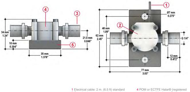
2 Completely encapsulated electronics
