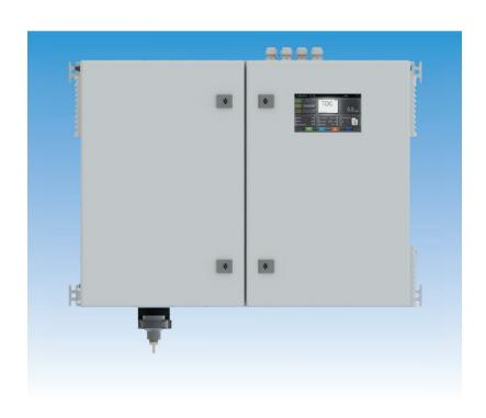
Online monitoring of total organic carbon is essential for regulatory and process control purposes among water treatment, wastewater and industrial users. Teledyne's 6700E Series employs proven UV-Persulfate methodology to isolate only organic carbons, oxidize them into carbon dioxide and measure TOC in the gas phase using infrared absorption technology. This method conforms to EPA, DIN, CE, ASTM and NAMUR regulations as well as meeting requirements of ISO and EN directives.
