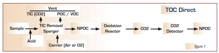
Acid is added to the sample, lowering its pH to approximately 2.0, at which point the carbonates present in the sample are converted to dissolved CO2.
