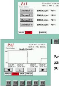
The instrument has an inbuild touch screen with functional keys that allows the configuration and manual control of the ISE-Analyzer. The results are displayed in numerical values for each channel or as a graph for a selected channel. Touch keys allow movement in the graph and zooming. In an additional window a table of the historical results is presented.
