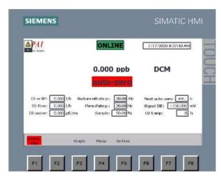
General control, Parameter setting and the visualisation of measurement results, messages as well maintenance requests are displayed on 7"-touch panel. menus password are protected to prevent unauthorized intervention. The screen displays measurement results numerically as well as graphically. For multiple
