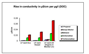
organic compounds in boiler and in the process of UV-treatment as performed by the **Organic X Monitor** *LC* is presented in the following figure. As can be seen the increase in conductivity for halogenated compounds is much higher than for halogen-free
